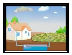
Rainwater harvesting is a technique used for collecting, storing, and using rainwater for landscape irrigation and other uses. The rainwater is collected from various hard surfaces such as roof tops and/or other types of manmade above ground hard surfaces.
